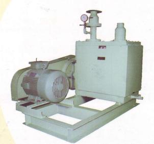
'RKHV' High vacuum pump is oil immersed rotary vane type. The main assembly consist of a main body with rotary vanes mounted eccentrically in it. The rotor is provided with two vanes opposite each other with springs in between which press them against the inner wall of the main body and make them move in and out of the rotor. The rotor revolves sweeping the air space twice each revolution.
